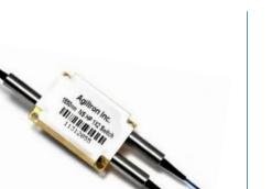
The NS 1x2 Solid-State Variable Fiber Optic Splitter splits an incoming optical signal among two output optical fibers with an electrically variable power ratio. This is achieved using a patent pending non-mechanical configuration. When the electrical control signal is removed, the splitter latches to a pre-determined ratio with a standard version of 100:0. The device is bidirectional, transmitting light in both direction simultaneously.
